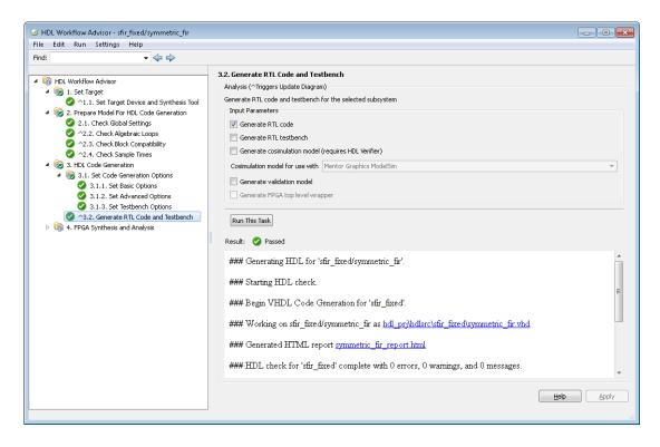
The code generation report, which includes the resource utilization and traceability reports, opens automatically. The resource utilization report shows the hardware resources your design implementation is using. The traceability report enables you to navigate between your model and the generated code.
