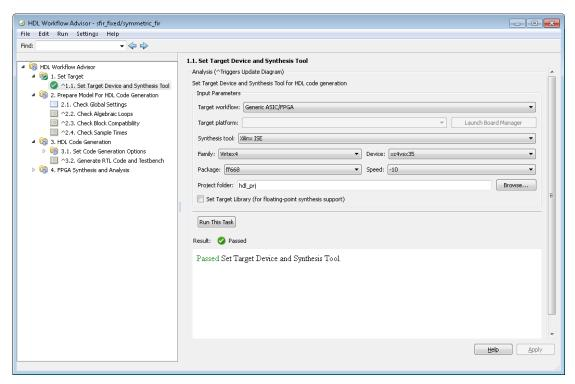
3 Right-click **Prepare Model For HDL Code Generation** and select **Run All**. The HDL Workflow Advisor checks the model for code generation compatibility.
