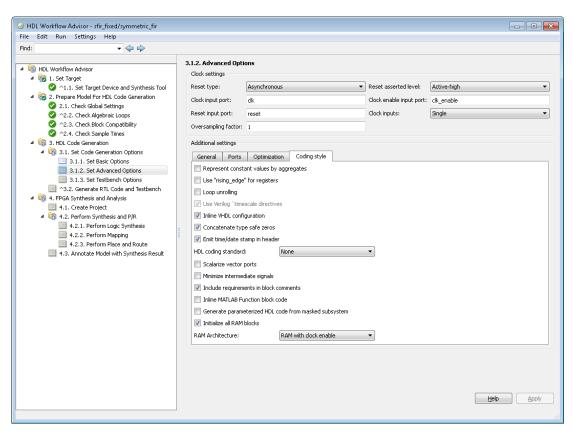
6 Right-click the HDL Code Generation > Generate RTL Code and Testbench step, and select Run to Selected Task.
