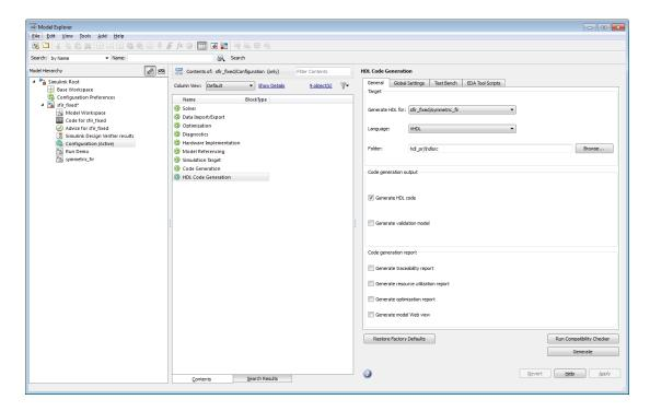
In the code generation exercises that follow, you use the Configuration Parameters dialog box to view and set HDL Coder options and controls. The exercises use the <code>sfir\_fixed</code> model (see "The sfir\_fixed Model" on page 2-16) in basic code generation and verification steps.
